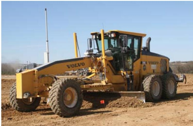
Schmidlein Excavating uses a Leica Power Grade 3D on a Volvo G940 motor grader.
